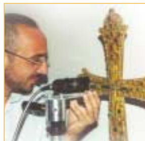
Renishaw's RP10 compact probe being used to analyse gemstones in situ
